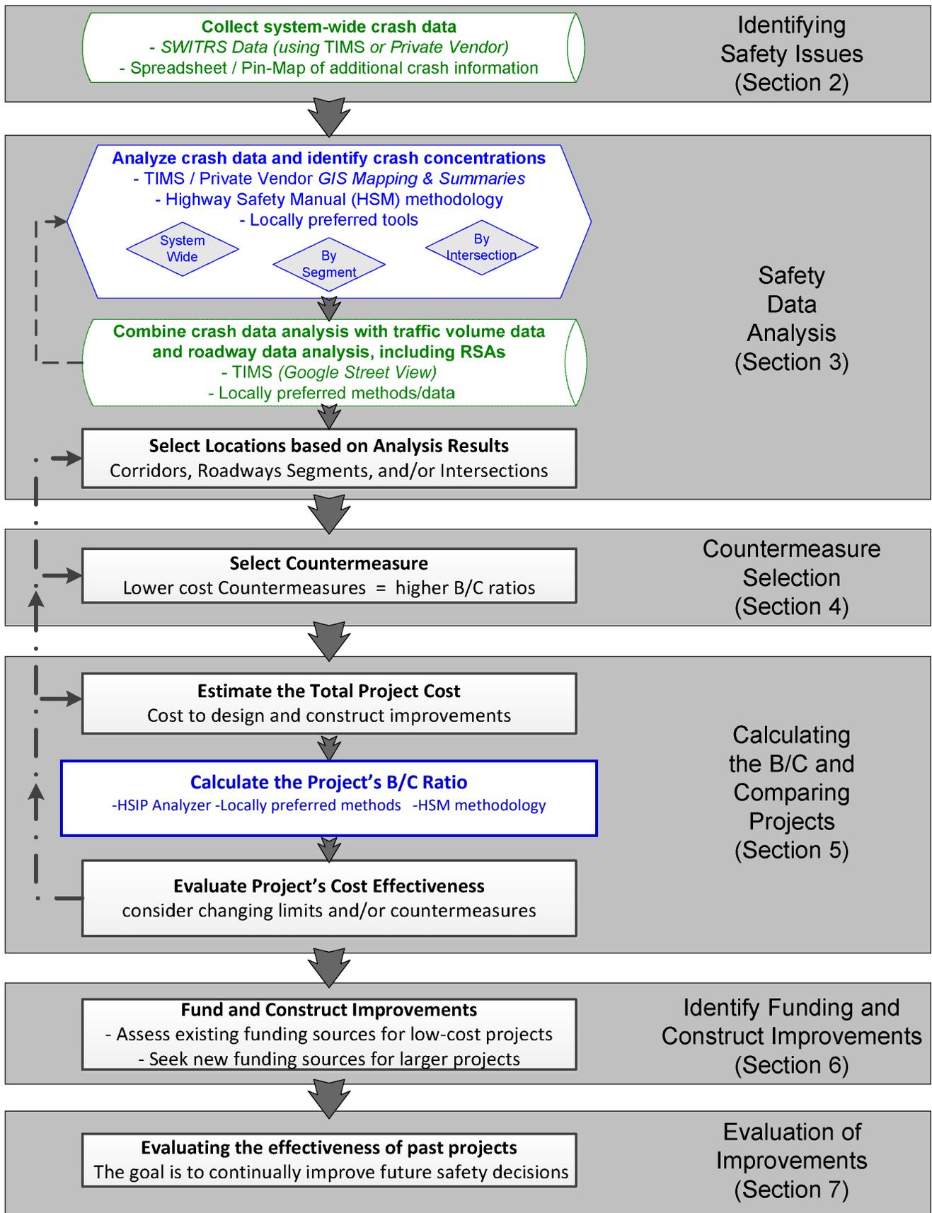
The above flowchart illustrates how each of the individual sections of this document work together to make up a proactive safety analysis approach. These sections are briefly outlined below:
