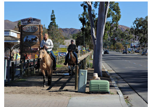
Equestrian trail physically separated from vehicular traffic by a split rail fence
