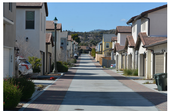
Residential alley provides garage and parking access, is used for trash pickup, and houses public utilities.
